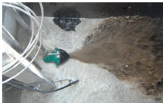
Rührdüse in Betrieb | Agitating nozzle in operation
